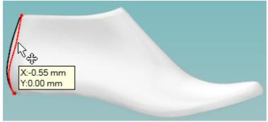
Scale - Allows to scale the line from template. Additional information about the line length is provided.
