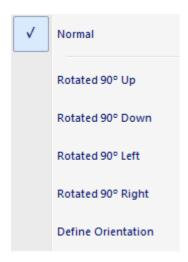
**Normal** - pivot axis is perpendicular to helper plane (ie. the accessory is placed as showed on the last surface)
