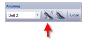
Activate **Manual alignment** from the **Aligning** toolbar. A reference system will appear with green handles on the axis. By default, the first interaction mode is **Move**.
