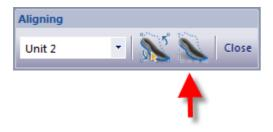
Activate the **Automatic alignment** button from the **Aligning** toolbar. A dialog will appear stating the four reference points needed for the process.
